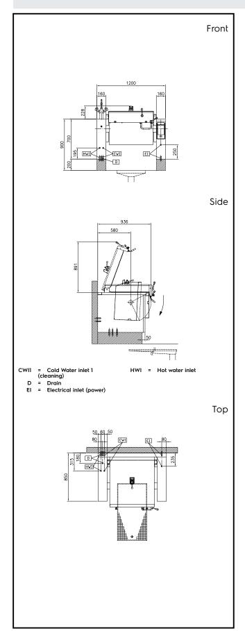
Electric Supply voltage: 400 V/3N ph/50/60 Hz Total Watts: 15.5 kW Installation: FS on concrete base;FS on feet;On base;Standing Type of installation: against wall **Key Information:** Working Temperature MIN: 50 °C Working Temperature MAX: 250 °C Vessel (rectangle) width: 680 mm Vessel (rectangle) height: 274 mm Vessel (rectangle) depth: 558 mm External dimensions, Width: 1200 mm External dimensions, Depth: 850 mm
